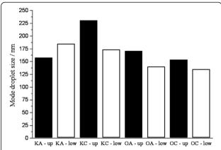
Figure 1 Mode droplet size values of different fractions of admixtures at the initial (without up or low index) point and after 24 hours.
